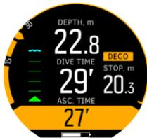
Suunto D5 shows the ceiling value always from the deepest of these stops. Deep stop and safety stop ceilings are always at constant depth when you are at the stop. Stop time is counted down in minutes and seconds.
