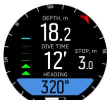
In the switch window, you see the heading in numeric format.
