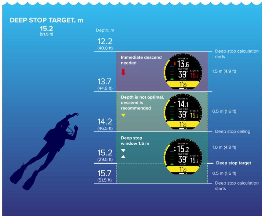
Below 20.0 m (65.6 ft), deep stop gets activated. In this case, as the diver ascends, the deep stop is necessary at halfway of the maximum depth, so at 15.2 m (49.8 ft).
