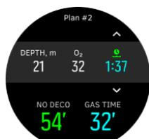
The calculated no decompression time is based on dive depth and gas mixture. Any residual nitrogen from previous dives, as well as surface time, is taken into consideration. **Gas time** is dependent on the dive depth, personal consumption and tank size/pressure.
