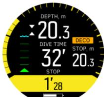
With decompression stops, the ceiling is always decreasing while you are near the ceiling depth, providing continuous decompression with optimum ascent time.
