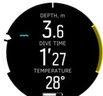
It is the default view. The white arrow on the left side of the arch moves according to the depth. The yellow arch shows the depth between the max depth (defined by Depth notify 5) and the next deepest active depth notification.
