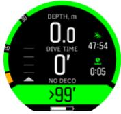
No-fly time is the minimum surface time after a dive which is recommended to wait before entering and flying with an airplane. It is always at least 12 hours and equals desaturation time when it is more than 12 hours. For desaturation times shorter than 75 minutes, no-fly time is not displayed.
