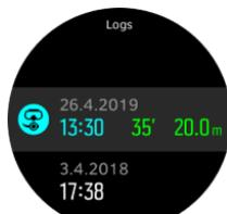
Dive log details and profile can be browsed by scrolling through the log with upper or lower button and selecting it with the middle button.
