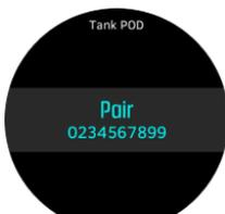
2. Make sure the Tank POD has been activated by ensuring there is tank pressure reading in screen and that it is within range. In the menu, the Tank POD is identified by the serial number printed on the Tank POD.
