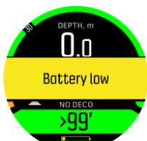
When the time left decreases to 2 (two) hours a 'Recharge needed' red pop-up notification appears. The red pop-up will stay on the screen on top of everything else and you cannot make it disappear until the device is charged or you change to time view. In case of scuba diving, when the charge level drops below 2 (two) hours, you cannot start a dive with Suunto D5. For freediving the limit is 30 minutes.
