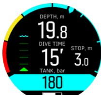
In the switch window, the actual tank pressure is shown in a blue field by default. This is also shown with a blue arrow in the arch. The blue part of the arch indicates the range between the value you set for the tank pressure alarm and the actual tank pressure:
