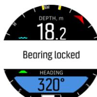
After you locked the bearing, you can see yellow bars to indicate the angle where you locked the bearing:
