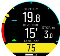
When the tank pressure drops below 50 bars (so within the red area in the arch) the actual tank pressure value is indicated in a red field in the switch window and a mandatory alarm is triggered:
