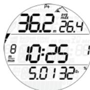
Press the button to scroll between the pages of information, press and hold the button to return to the list of main logbook menu. Inside the logbook menu, every 5 logs there is a page with **BACK** on the display, which allows you to leave the logbook menu by pressing and holding the button. Simply press when **BACK** is displayed to move on to the next dive in the logbook.
