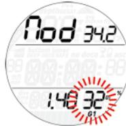
Once inside this menu, press the button to change the O<sub>2</sub>% and observe how this affects the maximum operating depth (MOD). Then press and hold the button to move on to the ppO<sub>2</sub>max and use the button to change the value, again noticing how this affects the MOD. Press and hold the button again to save the setting. To exit the menu, press the button until **bACK** appears on the display, then press and hold the button.
