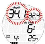
The alarm persists until the diver has ascended enough for the  $ppO_2$  to return within the set limit.
