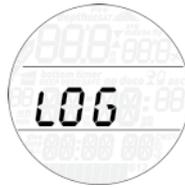
Puck Pro can record the profiles of approximately 35 hours of diving, at a sampling rate of 5 seconds. The information can be transferred using the optional USB clip to PC via the Dive Organizer software or to a Mac via the Divers' Diary software. In addition, Puck Pro can show most of the information directly on the display.
