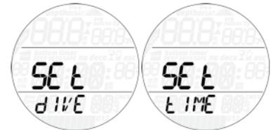
Press and hold the button to enter a menu, press the button to scroll up and down between available options or to increase or decrease the value of a setting. Then press and hold the button to confirm the change in setting. Press the button until you see **bACK** on the display then press and hold the button to go up one level in the menu tree.
