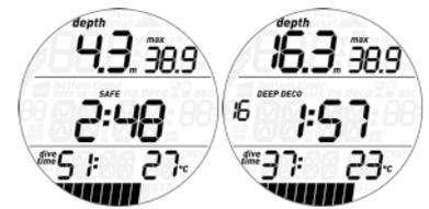
For **DECO** stops, since the duration is a function of the exact depth, only the minutes are shown.
