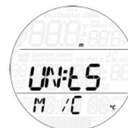
You can choose between metric (depth in meters, temperature in °C) and imperial units. (depth in feet, temperature in °F).
