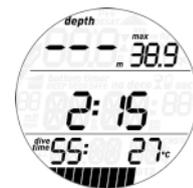
Upon returning to the surface, Puck Pro first goes into the so-called surfacing mode. This mode allows you to resume your dive after a brief period of orientation. The screen shows a 3-minute countdown.
