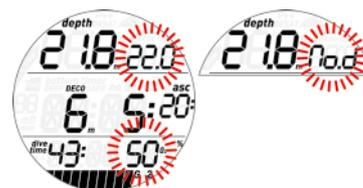
Press and hold the button to confirm the switch to G2, or simply press to cancel the gas switch and stay with G1. In both cases the set oxygen concentration will be displayed steadily in the lower right corner of the screen, and within 20 seconds the ascent time is updated to reflect the higher oxygen concentration in the breathing gas.
