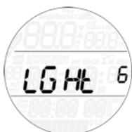
Puck Pro has a backlight which can be activated in case of low ambient light. The backlight is activated by pressing and holding the button. During a dive, the backlight will stay on for the duration defined in this menu. You can choose between 1 and 10 seconds, or you can set it to **on**. If you set it to **on**, the backlight will remain on until you press and hold the button again.
