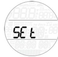
Puck Pro's **SEt** menu allows you to change settings. Once inside this menu, press the button to scroll between two submenus: **SEt dIVE**, where you can set parameters pertaining to the dive, and **SEt tIME**, where you can set parameters pertaining to time and date.
