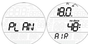
This function allows you to scroll through the no decompression limits, automatically taking
