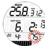
When the oxygen toxicity level approaches 100%. The alarm message and the audible signal are repeated for 5 seconds in one-minute intervals after the first occurrence and for as long as the value of CNS stays at or above 100%. Consider terminating the dive immediately!
