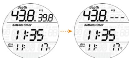
While the time of day is displayed, pressing and holding the button restarts the stopwatch.
