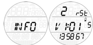
This submenu provides information about the hardware and software of your Puck Pro and about the status of the battery with a number from 1 to 3, 3 being the highest, 2 corresponding to a steady battery symbol and 1 to the blinking battery symbol (no dive).
