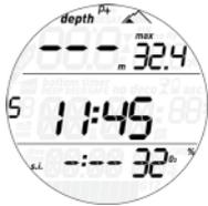
The pre-dive display shows p factor and altitude settings, time of day, surface interval since the last dive and temperature. If Nitrox is set, it will show the O<sub>2</sub> percentage and the corresponding MOD. A small S or F to the left of the middle row indicates the water type.
