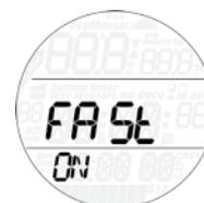
A fast (uncontrolled) ascent is defined as one in which a speed of 12 m/min / 40ft/min or higher was maintained over more than two thirds of the way up. This applies to dives deeper than 12m/40ft only. In such an event, due to the potential of harmful bubble formation, Puck Pro locks the computer for 24 hours in order to discourage you from diving again. In this menu, you have the option to disable the locking up of the computer in the event of an uncontrolled ascent.
