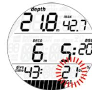
Press the button while this indication is blinking to initiate the gas switch: the oxygen percentage of G2 starts to blink in lieu of that of G1, and in the top right corner the letters MOD and the value of the MOD for G2 alternate every 2 seconds.
