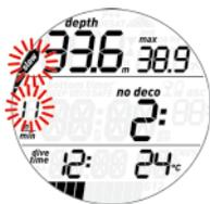
If the ascent rate exceeds 12m/min / 40ft/min at a depth below 12m / 40ft, the blinks as well. If a speed in excess of 12m/min / 40ft/min is maintained for two thirds or more of the depth at which the alarm was first triggered, Puck Pro considers it a dive violation and the display will show the steady symbol.
