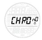
Press and hold the upper button to enter this menu. The middle row now features a stopwatch while the time of day has moved to the bottom row. Press the upper button to start and stop the time, then press the lower button to reset the time to zero. Press and hold the lower button to exit from the stopwatch function (this stops and resets the stopwatch if it was running or stopped at a non-zero value upon exiting).
