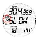
In this case, if the diver attempts a repetitive dive after surfacing, Smart will only function as a depth gauge and timer (bottom timer mode), *SLOW* and will display *DOWN*: on the screen throughout the dive.
