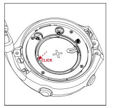
g) Position the new o-ring from the kit in the groove around the battery, ensuring that it sits towards the outer edge of the groove.
