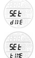
Press and hold the upper button to enter a menu, then press either button to scroll up and down between available options or to increase or decrease the value of a setting. Then press and hold the upper button to confirm the change in setting. Press and hold the lower button to go up one level in the menu tree.
