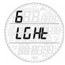
Smart has a backlight which can be activated in case of low ambient light. The backlight is activated by pressing and holding the lower button. During a dive, the backlight will stay on for the duration defined in this menu. You can choose between 1 and 10 seconds.
