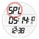
The stopwatch features also a split-time function: by pressing the lower button while the stopwatch is running, the time itself will freeze while **SPL** blinks in the top row and the stopwatch continues in the background. Every time you press the lower button the split time will refresh with the new value. Press and hold the lower button to exit the split-time mode. Note that while in split-time mode, the upper button has no function.
