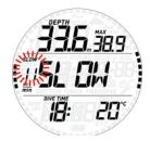
If the ascent rate exceeds 12m/min / 40ft/min at a depth below 12m / 40ft, **DOWN!** appears and the speed value blinks. If a speed in excess of 12m/min / 40ft/min is maintained for two thirds or more of the depth at which the alarm was first triggered, Smart considers it a dive violation and the display will show the steady **SLOW DOWN!** symbol.
