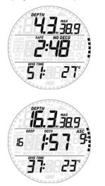
For **DECO** stops, since the duration is a function of the exact depth, only the minutes are shown.
