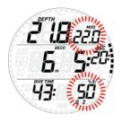
Press and hold the upper button to confirm the switch to G2, or press the lower button to cancel the gas switch and stay with G1. In both cases the set oxygen concentration will be displayed steadily in the lower right corner of the screen, and within 20 seconds the ascent time is updated to reflect the higher oxygen concentration in the breathing gas.
