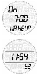
Smart features a "sleep" mode: in case you don't wear it other than on a dive trip, you can put Smart in sleep mode to reduce battery consumption. To wake up from sleep mode, press either button.
