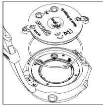
Remove the battery by prying it loose with a small flat-head screwdriver.
