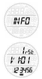
This submenu provides information about the hardware and software of your Smart and about the status of the battery (two segments inside the battery means the battery is ok, one segment means the battery is low but the watch functions as dive computer, one segment blinking means the battery is too low for use as dive computer).
