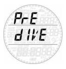
Press and hold the upper button to enter this menu and put Smart into the ready-to-dive mode.
