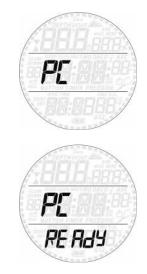
This submenu allows you to download your dive data to a PC or Mac. Press and hold the upper button and the display will show **PC ready**, symbolizing that Smart is ready to communicate.
