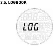
Smart can record the profiles of approximately 35 hours of diving, at a sampling rate of 5 seconds. The information can be transferred using the optional USB clip to PC via the Dive Organizer software or to a Mac via the Divers' Diary software. In addition, Smart can show most of the information directly on the display.
