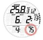
When the oxygen toxicity level reaches 100% the alarm message and the audible signal are repeated for 5 seconds in one-minute intervals after the first occurrence and for as long as the value of CNS stays at or above 100%. Consider terminating the dive immediately!
