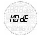
Here you can define the type of gas you will be breathing during the dive (air or enriched air nitrox, including multigas). You can also set Smart to bottom timer, in which case Smart will show only time, depth and temperature: it will not carry out any decompression calculation and it will not show any warnings and alarms. You can set Smart also to freediving mode, which in essence is a bottom timer with special features dedicated to free divers.
