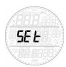
Smart's **SEt** menu allows you to change settings. Once inside this menu, press either button to scroll between two submenus: **SEt dIVE**, where you can set parameters pertaining to the dive, and **SEt tIME**, where you can set parameters pertaining to time and date.
