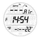
The pre-dive display shows p factor and altitude settings, time of day, surface interval since the last dive and temperature. If Nitrox is set, it will show the  $O_2$  percentage and the corresponding MOD. A small S or F to the left of the middle row indicates the water type.
