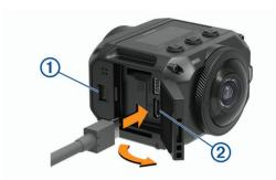
3 Plug the small end of the USB cable into the micro-USB port
