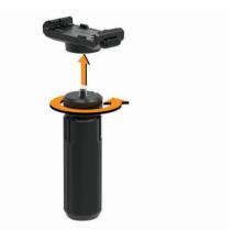
2 Place one side of the camera into the cradle, fitting the grooves in the side of the camera onto the teeth.
