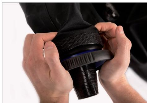
**2.1** Grab the seal in a firm grip so that it don't slip out of its position while you press the assembly into the PU-Ring on the drysuit. Push the assembly into the PU-Ring until the back-end of the assembly has passed the front end of the PU-Ring.
