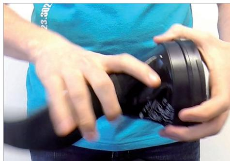
**4.6** Test the strength of attachment by pulling VIRGO Ring and glove in the opposite direction. If the assembly does not hold together, please change the Spanner Ring to a thicker one.
