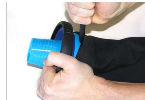
**3.1** Use the Combi Tool to detach the VIRGO assembly from the PU-Ring in your drysuit. Push the lever of the Combi Tool into a groove and pry out the VIRGO assembly.
