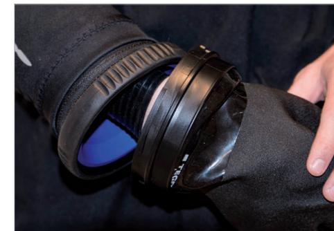
**5.2** Join the rings together (make sure that the O-ring and sealing surface are properly cleaned and lubricated).
