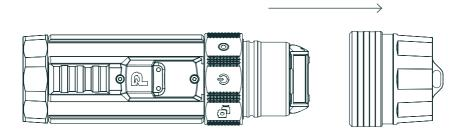
To put the end cap back on, pull back the lock ring on the end cap, and push the end cap back on.
