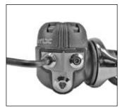
3. Check to ensure the o-ring is present and in good condition. Screw the threaded end of the hose into the port and tighten to 40 in-lbs (4.5 Nm) with a 9/16" wrench
