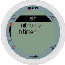
Use the buttons on the right side to highlight your choice, then press and hold the top right button to activate it. **air** is the equivalent of setting **nitrox** to 21% and a  $ppO_2max$  of 1.4bar, but simplifies the display a bit by not showing the CNS (its value however is calculated in the background and if needed the 75% warning and the 100% alarm are triggered).
