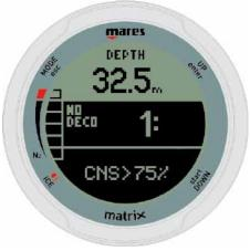
When the oxygen toxicity level approaches 100%, the alarm message **CNS > 100%** appears. The alarm message and the audible signal are repeated for 5 seconds in oneminute intervals after the first occurrence and for as long as the value of CNS stays at or above 100%. Consider terminating the dive immediately!
