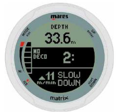
If the ascent rate exceeds 12m/min / 40ft/minat a depth below 12m / 40ft, the message on the screen changes to **TOO FAST**. If a speed in excess of 12m/min / 40ft/min is maintained for two thirds or more of the depth at which the alarm was first triggered, Matrix considers it a dive violation and the display will show  $\Delta$ .
