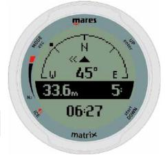
By pressing and holding the bottom right button you activate the stop watch. This can be helpful when timing yourself on the leg of a navigation course. Every time you press and hold the bottom right button, the stop watch restarts from 00:00. If you exit the compass the stop watch keeps running in the background.
