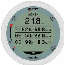
Matrix always begins the dive with G1, which has the lowest percentage of oxygen. When during the ascent you reach the depth corresponding to the MOD of G2, Matrix sounds an audible signal and displays the message GAS 1 -> GAS 2 at the bottom of the screen.
