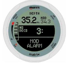
The alarm persists until the diver has ascended enough for the  $ppO_2$  to return within the set limit. While the alarm is active, the compass can only be called up for 8 seconds, after which the default display with the alarm message is shown again.
