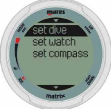
Press and hold the top right button to enter a menu or submenu, press the right side buttons to scroll up and down between available options or to increase or decrease the value of a setting. Then press and hold the top right button to confirm the change in setting. Press or press and hold the top left button to exit a menu without saving the last change.
