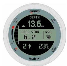
DEEP stops are generated as you approach the no deco limit. You can either have one 2-minute stop or two 1-minute stops. DEEP stops are NOT mandatory.
