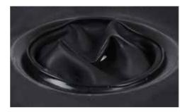
**1.5** Press with you fingers/with the Combi tool all around, until the Lock Ring and seal assembly has been forced into the groove in the Neck Ring. (Strive to get the same amount of excess part of seal around the entire assembly, see image **1.6.**)
