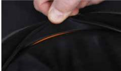
**1.7** Check that the Lock Ring is in position by following the groove 360°.
