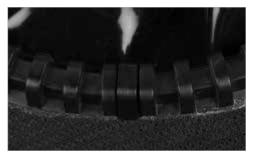
**2.5** When clip is installed correct it should sit as in above picture.
