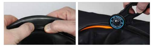
**1.3-1.4** By applying force, press the Lock Ring down into the tapered groove of the Neck Ring so that the Lock Ring enters the groove and locks into position. This can be done either with the force of your fingers or by using the Combi tool.
