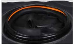
**1.1** Place the Lock Ring on the inside of the seal. Ensure that approximately 1,5 cm of the seal is pulled over the Lock Ring.
