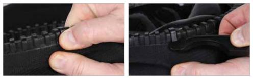
**3.1** Press with your thumb on the flat surface under the clip that you want to remove. Lift the bottom part of the clip with your other hand and fold the clip up- and backwards. If the clip is hard to remove by hand, you may use a tool to lift the clip up- and backwards. (For example the Combi tool, a screwdriver or other tool that has a flat and blunt edge.)
