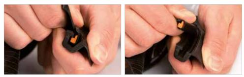
**3.3** The ORUST Neck Ring is designed for dynamic flexibility and will not demand tools for release of the Lock Ring and seal. You can easily release the Lock Ring by using your fingers. Grab the neck seal with one hand and bend (open) the ORUST Neck Ring with the other hand. Pull firmly until the seal and Lock Ring comes loose. **NOTE:** Be aware of the fact that sharp finger nails might damage the seal.
