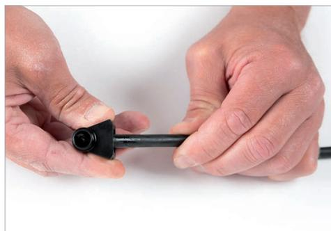
**2.4** The best way to get the cable through the swivel socket is to rotate the cable while pressing it forward into the socket. You may simplify this procedure by using a tool with soft edges! Do not use sharp tools as knives or similar as you may damage the socket or the cable.
