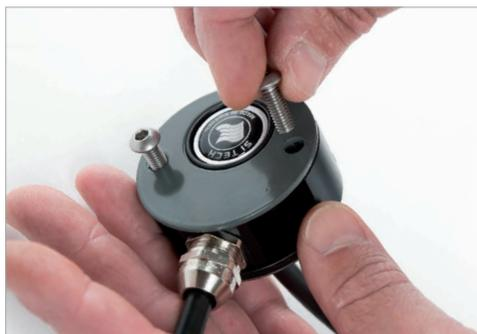
**3.3** Put the cover lid in position. Use your fingers to mount the screws and rotate them as far as you can by the force of your fingers. The Allen key must only be used when tightening the screws. Use gentle force when tightening the screws.
