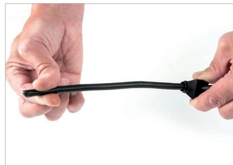
**2.5** Before next step it is important to measure the length of the cable for your specific need. When the nipple is mounted and fastened it will not be possible to adjust the cable in any direction without disassembly.
