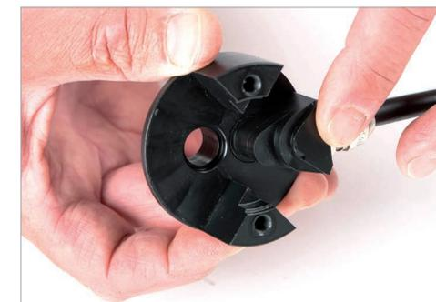
**2.8** Before you press the swivel into the bottom of the O-ring seat, the O-rings may need to be greased (preferably with silicone grease). Check the function of the swivel!
